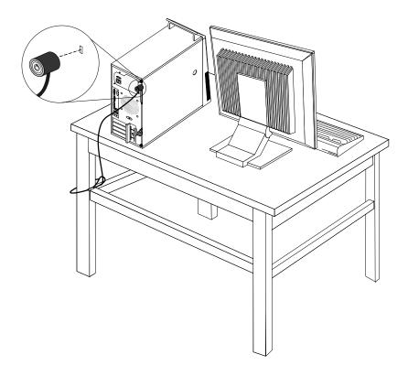
Figure 8. Integrated cable lock
